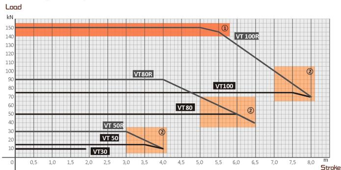
To ensure stability in the upper portions of the operating ranges, the VT Chain's drive system uses special components, in particular a double—key or splined shaft and longer drive guides. For loads above this limit, the drive system is equipped with a double—key or splined drive shaft. For strokes above this limit, the drive system is fitted with long drive guides.
